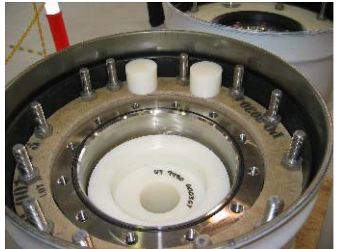
S-300 pipe overpack containers with neutron shielding material inside 200L drums.
