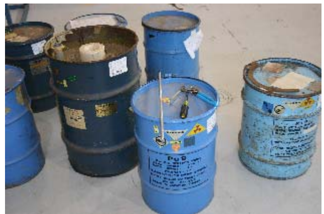
A selection of Pu-239/Be sources in original containers.
