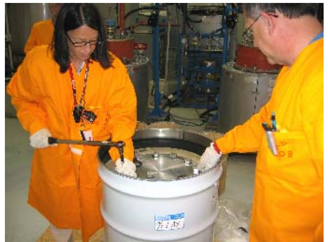
Sealing of overpack containing encapsulated Pu-239/Be source.
